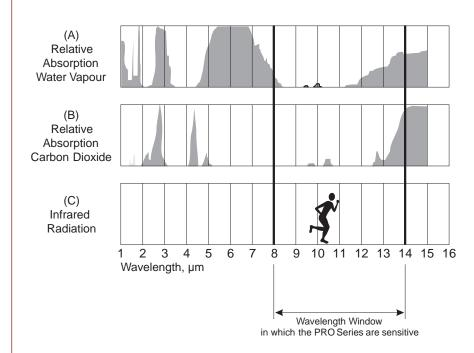
The wavelength of infrared absorption of primary atmospheric constituents compared to the wavelength of infrared radiation produced by humans
